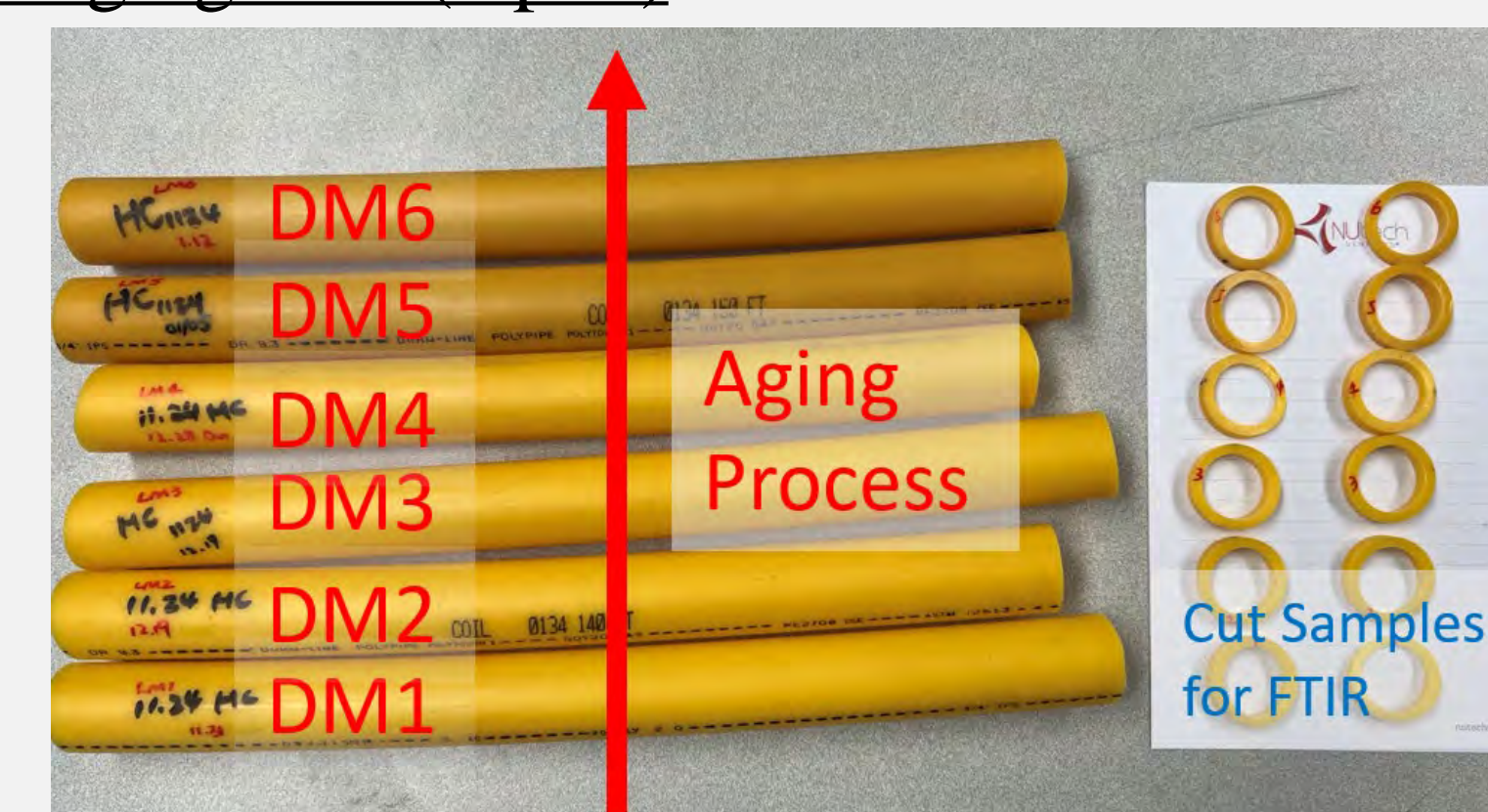
MDPE plastic's surface morphology vision inspection
