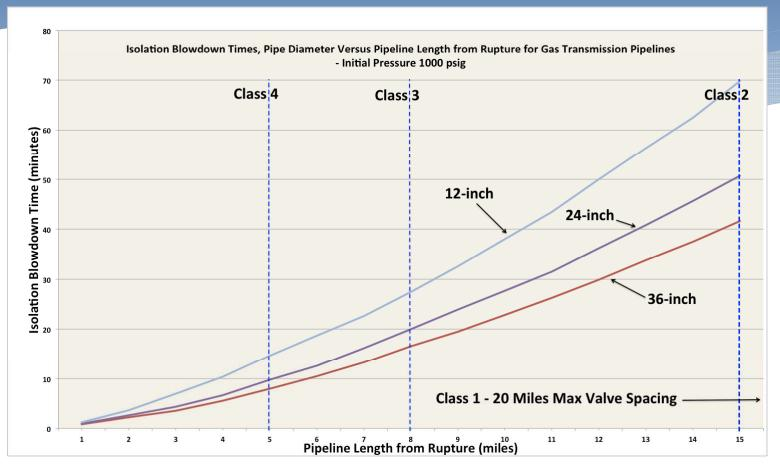
Isolation blowdown = time to vent after valve closed
