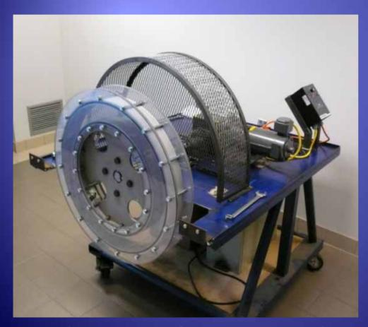
Simulates energy of mixing and particle collisions between solids flowing in slurry
