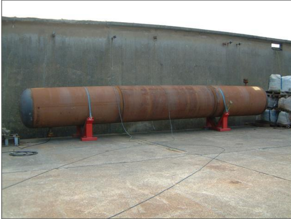
Fabricated Vessel with Machined Defect Located at Center of Vessel
