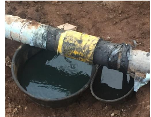
Figure 5: Failure at Dent under Composite Repair Sleeve
