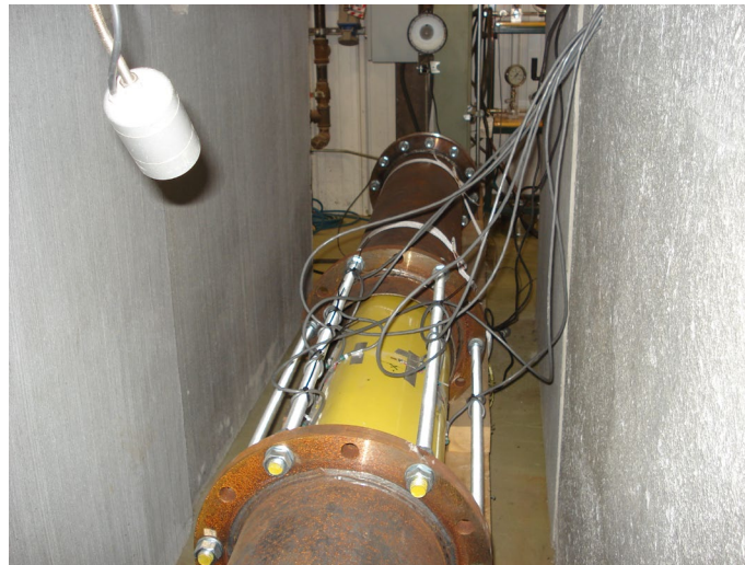
Bending, Pressure, and Permeability Testing of Liners
