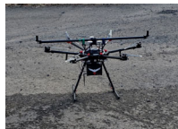
DJI Matrice 600 Pro equipped with the RedTail RTL-400 LIDAR System
