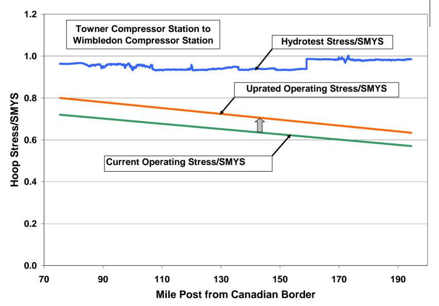
Effective test factor varies with elevation and distance from C/S discharge
