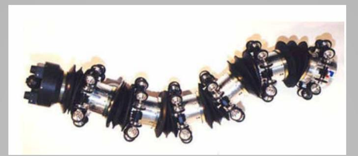
Video camera in head sends pictures to remote monitor. Future version to have supervised autonomous operation modes. Operator in control room could zoom in on pipeline features.
