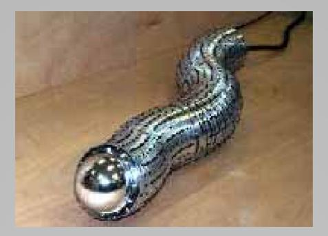
Tethered robot. Wide range of motion controlled by compressed air.
