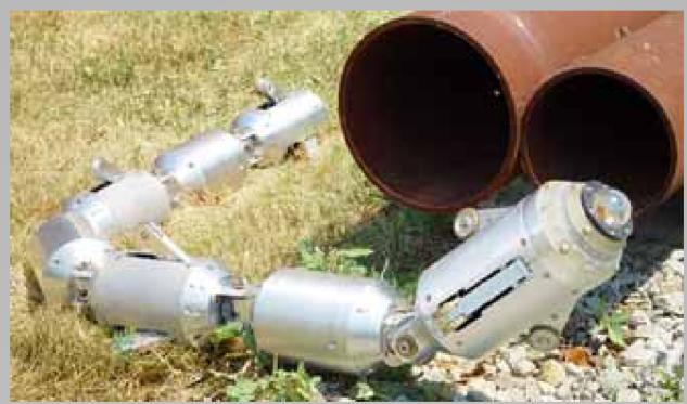
The locomotor module houses a mini fish-eye camera and lighting elements. The camera has a 190-degree field of view and provides high-resolution color images of the pipe's interior.
