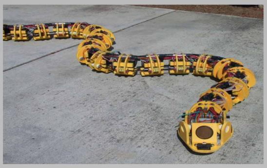
Dr. Gavin Miller prototype. Movement without wheels allows for rectilinear motion. Has bidirectional packet-based radio and a variety of sensors.
