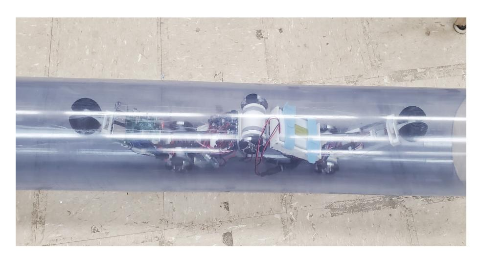
Figure 1. Sensing robot moving in a 6-inch pipe
