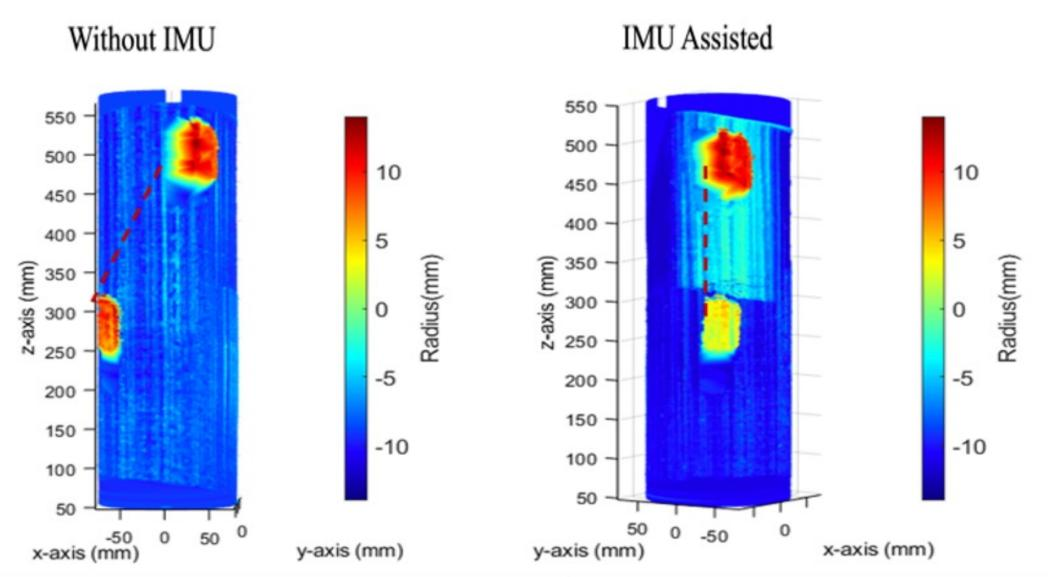
Figure.6. Proposed registration approach for sensor Figure.7. Side view of reconstruction pipe at 25-degree stabilization with data acquisition procedure rotation: without IMU (left) and with IMU (right).
