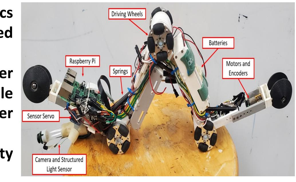
Figure 3. Designed robotic platform.
