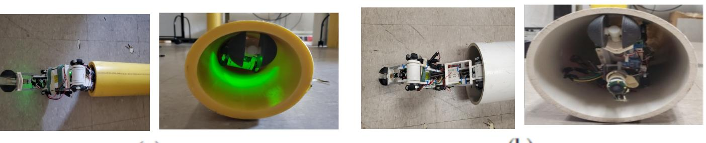
Figure 5. Robotic Sensing system in a) 4inch pipe view b) 6inch pipe view Feature-based registration with IMU and robot odometry assisted reconstruction
