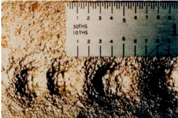
Cup-type scooped out hemispherical pits on flat surfaces with craters in pits
