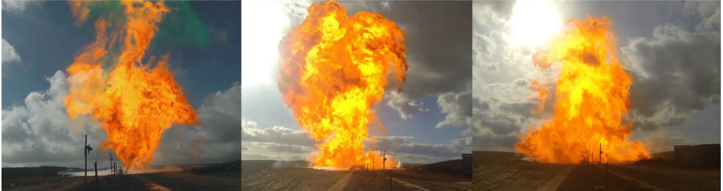
Figure 4: Induced LNG BLEVEs three seconds after rupture of the 5 m 3 vessels; Left - Experiment 2 (37% fill, 13 barg), Middle - experiment 3 (67% fill, 6 barg), Right - experiment 4 (69% fill, 13.6 barg).
