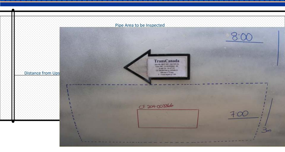
Marking out pipe for inspection – keeping in mind specific ILI Tool's tolerances PHMSA Crack Management Workshop | Chicago | August 5, 2014
