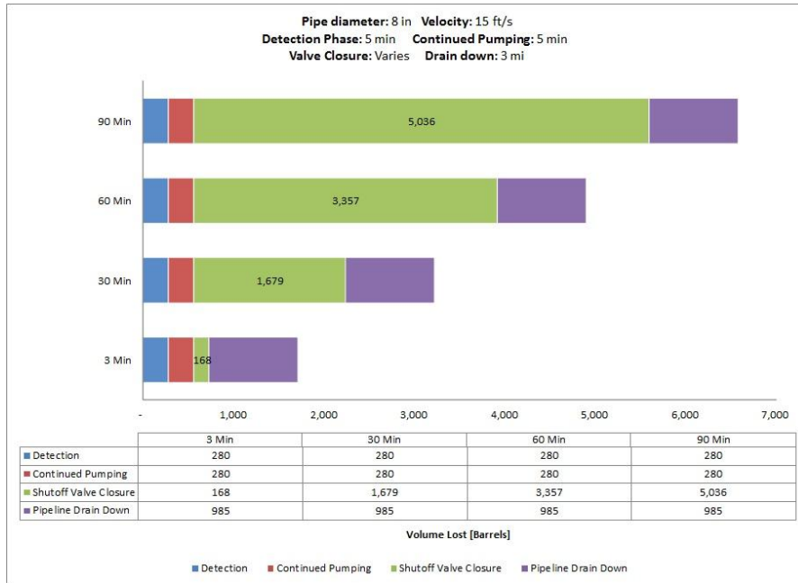
Fig. 3.81. Case Study 7D – Discharge volumes for an 8-in. hazardous liquid pipeline with a 1,480 psig MAOP and an elevation change of 1,000 ft with a 3, 30, 60, and 90 minutes block valve closure phase.
