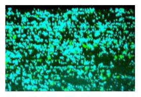
Epifluorescent and phase contrast microscopy relate bacteria to corrosion on the coupon; staining protocols used to identify specific bacteria types
