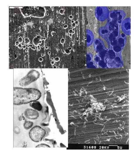
After various exposure periods, the coupons were preserved, embedded and examined using phase contrast and UV fluorescence microscopy, transmission electron microscopy and scanning electron microscopy.
