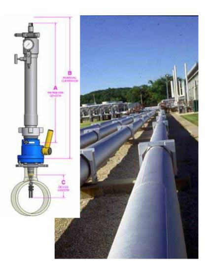
Extended analysis coupons (EM coupons) are exposed to process fluids in the same manner as weight loss coupons
