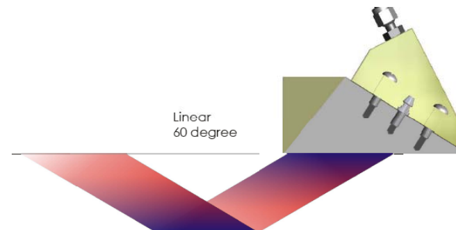
Figure 5 Linear PA Beam Pattern Example
