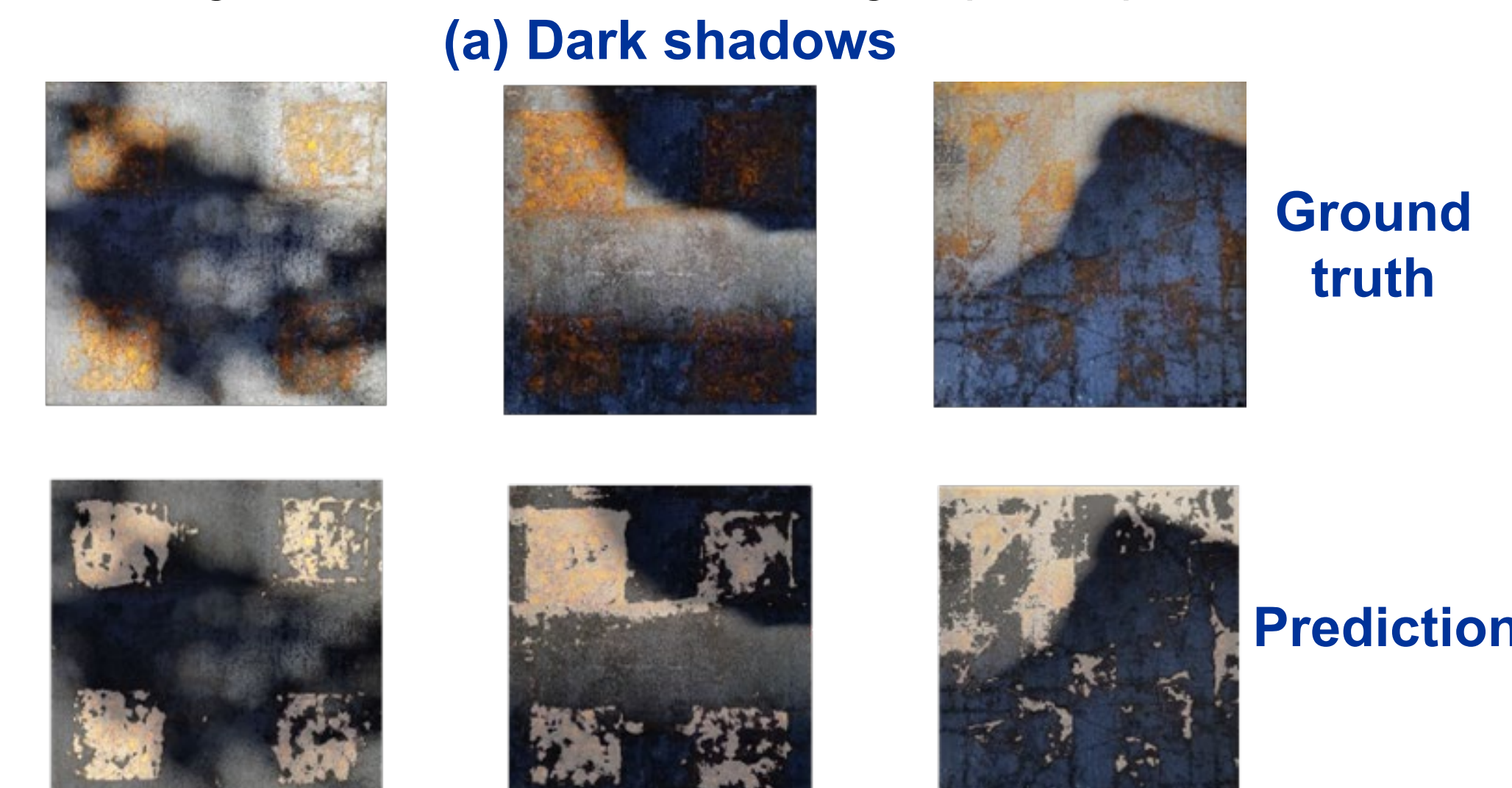
Fig 7: In-lab validation of the trained ANN to identify corrosion under (a) dark shadows and (b) illuminations.
