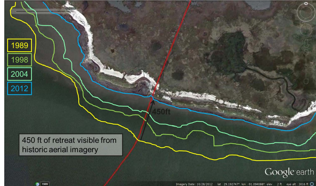
Coastal retreat occurring in Gulf of Mexico. Visible retreat of 450 ft over past 25 years (Louisiana).
