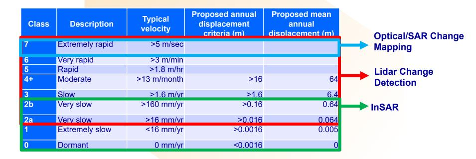
Overlapping Levels of Detection (LoD) / Limitations Point To the Benefit of Combining Several Methods to Characterize the Ground Displacements of Interest to Pipeline Integrity Management.
