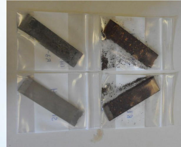
Test coupons are 75 x 19 mm and 3 mm thick
