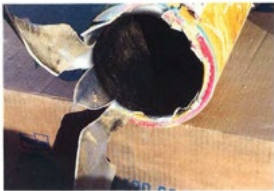
Figure 12. Leading Edge of Side B Clock Spring Arrestor After Test 6-1.
