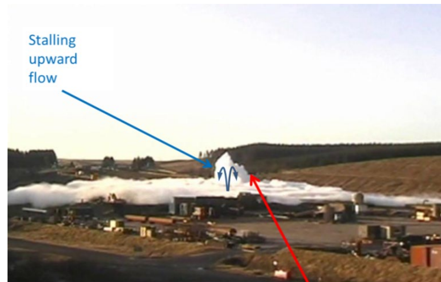
Crater is covered by vapour blanket – mixture released previously is drawn into flow
