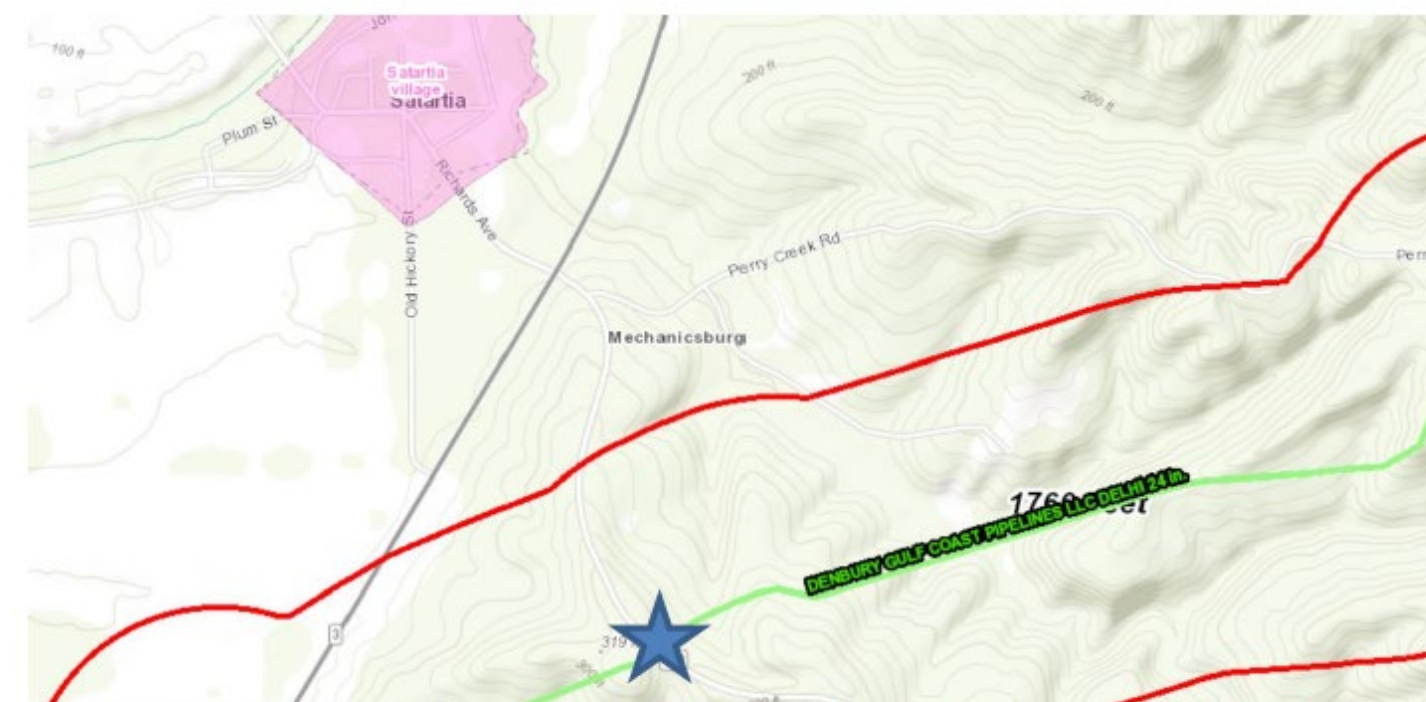
Figure 6: Topographical Map Showing the Delhi Pipeline (Green) and Denbury's Buffer Zone (Red) on Either Side of the Pipeline and the Proximity to Satartia (Blue Star Indicates the Rupture Site)
