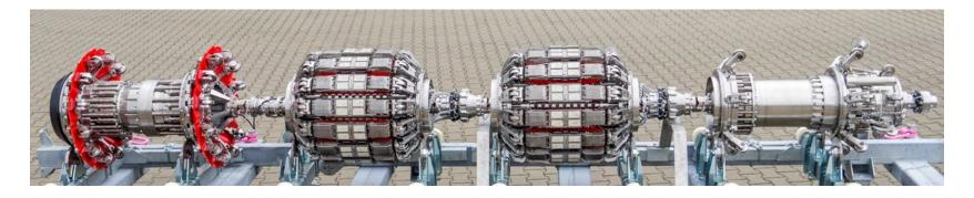
EMAT Ultra – development of EMAT technology (TRL5) includes miniaturization of sensors, send/receive from both sides and 200% coverage
