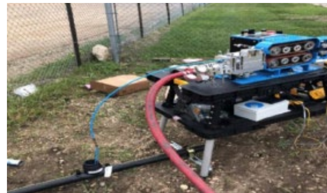
Prototype Testing of Pneumatically Driven Duct Rod Pusher Propelling Duct Rod into a Pipeline. Picture courtesy: Gas Technology Institute.
