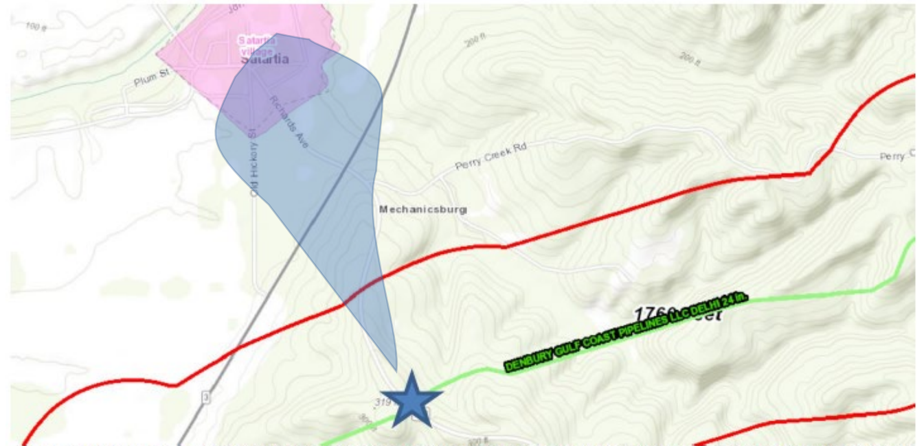
Figure 6: Topographical Map Showing the Delhi Pipeline (Green) and Denbury's Buffer Zone (Red) on Either Side of the Pipeline and the Proximity to Satartia (Blue Star Indicates the Rupture Site)
